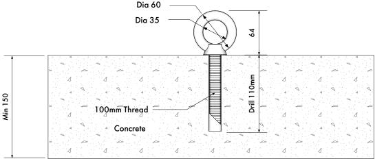
Use an Acrylic Epoxy (HILTI RE 500 or Equivalent) Chemical 2 pack compound to set anchor into concrete. (Approx 20ml per hole)
