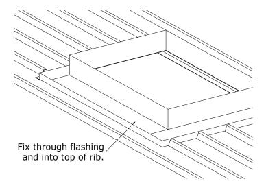
Fix front of hatch through front of flashing and into rear flashing up stand using rivets.
