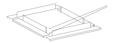
Flashing can now be riveted together. Apply more silicone over rivets if need be.
